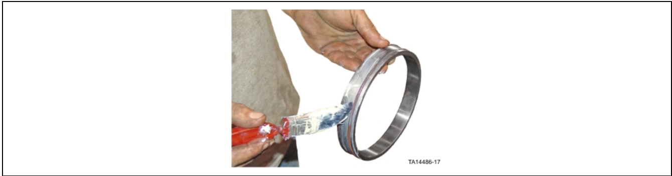
Figure 39. Application of assembly grease to sleeve O-ring and sleeve.
