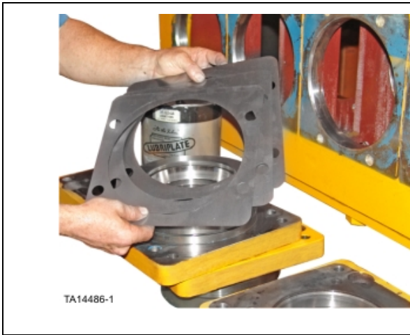
Figure 22. Three .020 shims to be installed to rear output bearing housing
