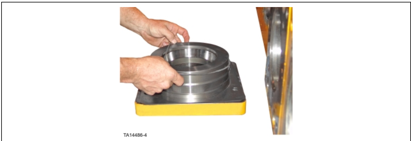
Figure 24. Installation of O-ring to rear output bearing housing
