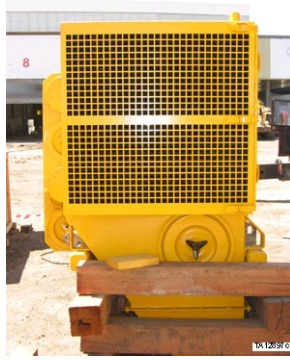
Figure 20. KLENZ™ and blower assembly supported by cribbing - 3 of 3
