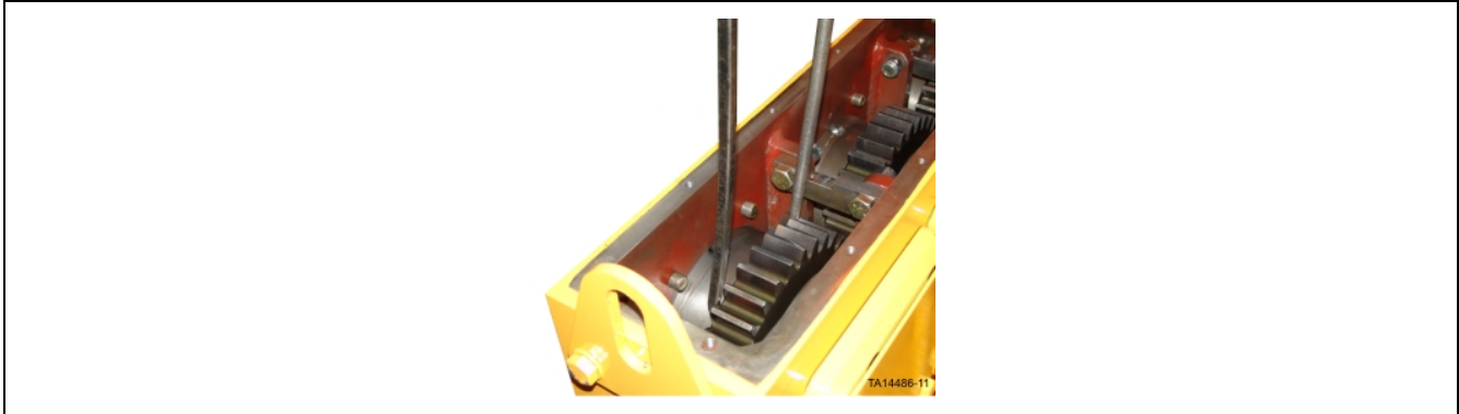
Figure 31. Gear pried toward rear of gearbox to measure bearing end play
