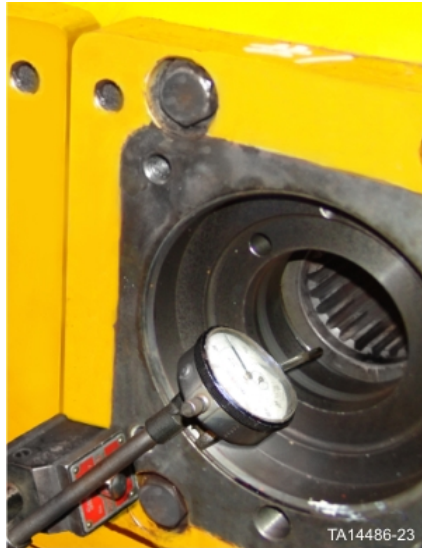
Figure 29. Magnetic base dial indicator in position to read bearing end play
