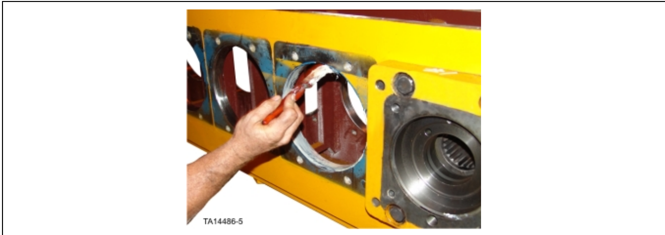
Figure 25. Application of assembly grease to gearbox
