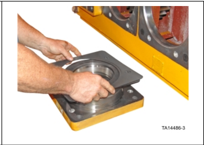
Figure 23. Installation of shims (.060) to rear output bearing housings
