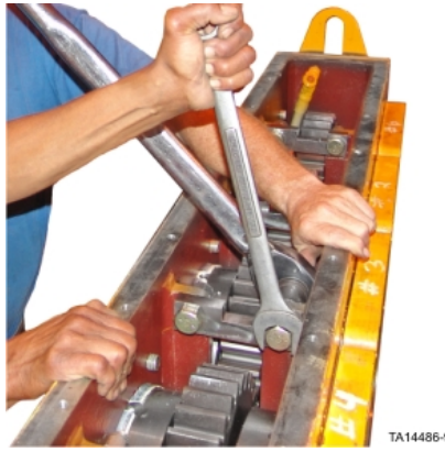
Figure 28. Installation of brace bars
