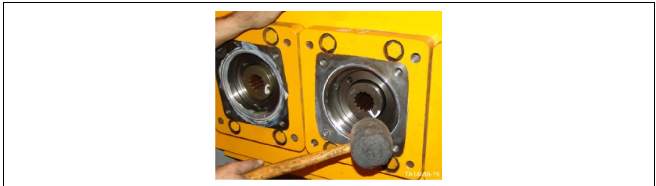
Figure 41. Installation of sleeve into output bearing housing
