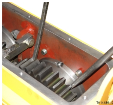
Figure 30. Gear pried toward rear of gearbox
