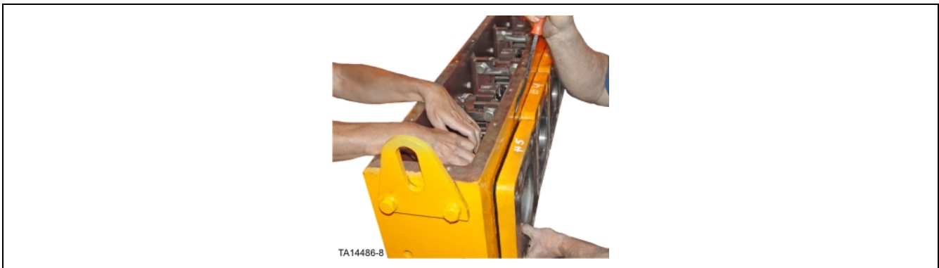
Figure 32. Removal of front output bearing housing for shim adjustment
