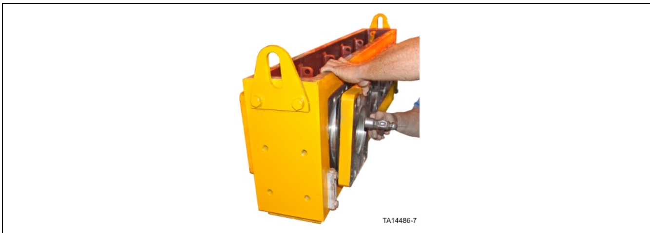
Figure 27. Installation of front output bearing housing with .040 shims in place
